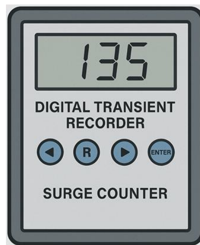
Gambar 3. Contoh Tampilan Alat Ukur Digital Transient Recorder/Surge Counter
