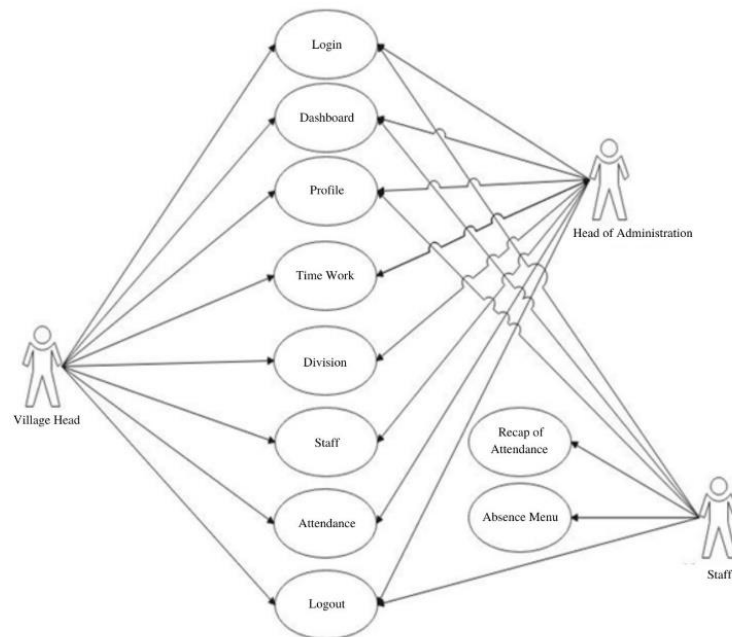
Figure 3. Use Case Diagram of Designing An Information System For Employee Attendance At The New Hapesong Village Office Web-Based
