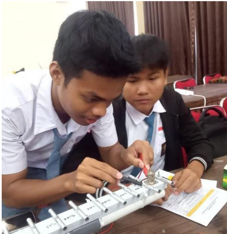
Figure 2. Participants assembling Yagi and conducting antenna performance measurements during the training session.
