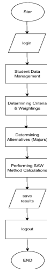
Figure 2. Admin system flowchart. (Source: Developed by the Author)
